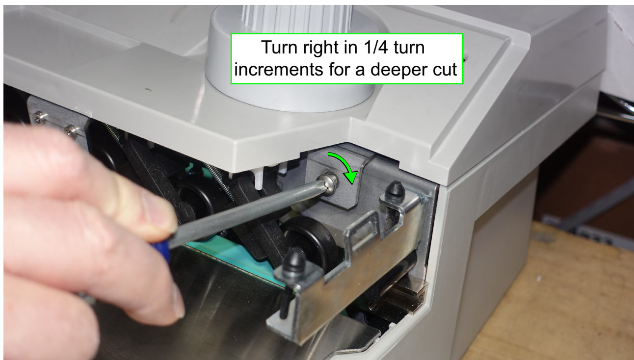
Figure 4-18: Adjusting the cutter depth
